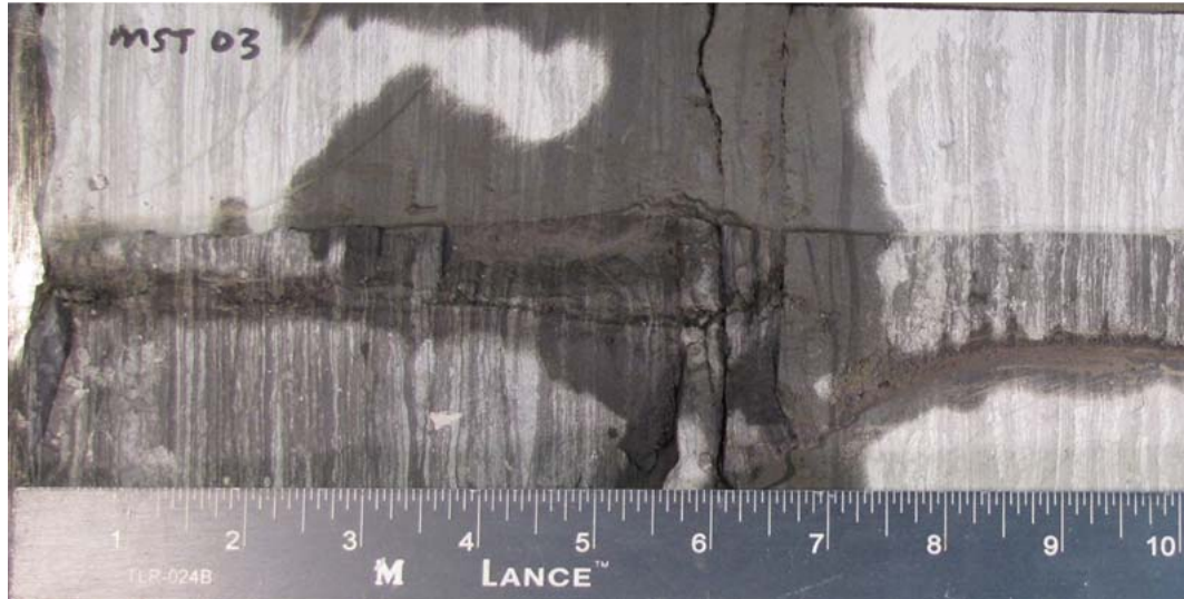
Figure 8: Conventional 15g Charge in Mancos Shale
