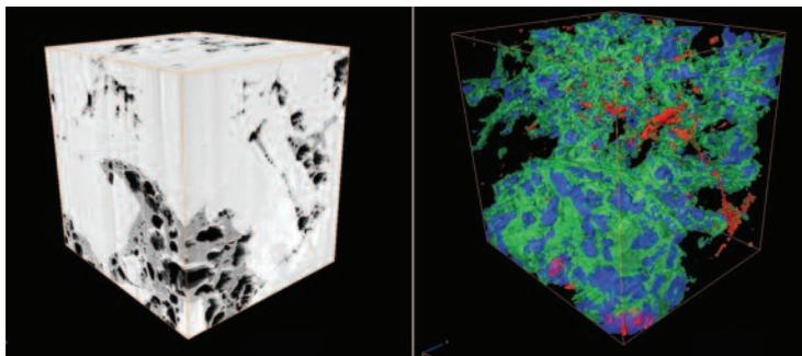
The image on the left shows the outer surface of a 3-D FIB-SEM volume from an organic-rich shale. The image on the right shows a transparency view of the distribution of connected pores (blue), isolated pores (red), and organic matter (green).
