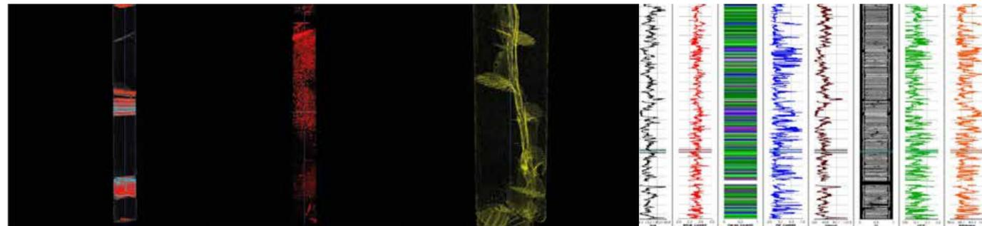
Figure 1. Visualization generated from whole core CT showing geologic features captured within the digital record (left). All data is managed in Lithovision™ where loading of all volumes based on petrophysical data is simple (right).
